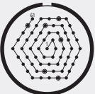
Arrangement 37-961 61 contacts size/taille 22
