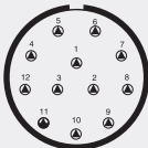
Arrangement 37-3 * 12 contacts size/taille 12
