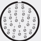
Arrangement 37-924 * 24 contacts size/taille 16
