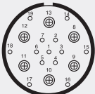
Arrangement 37-19 * 13 contacts size/taille 20 6 contacts size/taille 8
