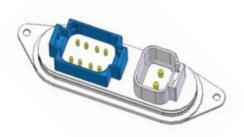
Flange receptacle including DT04-8P gold plated and DTP04-2P for power application to be integrated in an ECU. The flange is sealed to the unit housing.
