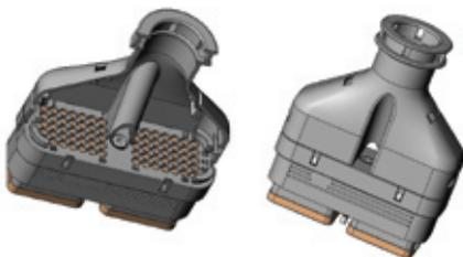
The innovative design of the DRC 70 pin wire router and corresponding back shell assures permanent access to the jackscrew for easy assembly and disassembly. The wire router allows optimized wire routing while the back shell includes a tie-wrap option for various harness diameters.
