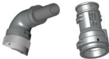
The Back Shells are designed to fix onto the connector modifications L017 of HDP size 18 and 24. The variety includes straight (180°) and right angled (90°) adaptors. The units fits to plugs and receptacles and accommodate several different sizes of slit or unslit corrugated tubes in the same back shell.
