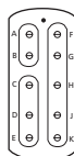
Disposition 20-10 1 circuit de/bus of 2 contacts 1 circuits de/bus of 3 contacts 1 circuits de/bus of 5 contacts taille /size 20
